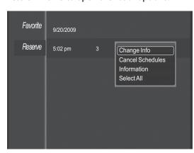
**5** Press ▲ or ▼ to highlight **Change** Info, then press **ENTER**. The *Timer Viewing* screen opens and displays the revered program information.
